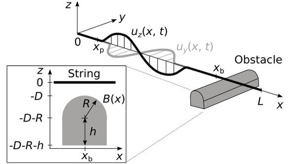
Figure 1: Schematic of the monochord. String length is  $L$ . String is excited at  $x = x_p$ . Rigid obstacle with circular cross-section is placed at the distance  $D$  from the string at its rest and at  $x = x_b$  along the string extent.
