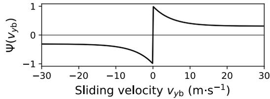
Figure 2: Friction characteristics curve where  $\beta = 0.20 \text{ s}\cdot\text{m}^{-1}$  and  $\psi = 0.45$ .
