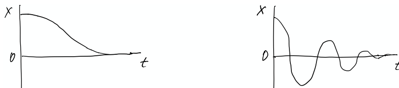
Figure 19: Comparison of a critically damped system solution time-series shown on the left to a damped system solution time-series shown on the right.
