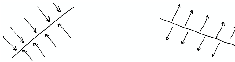
Figure 16: Phase portrait of non-isolated fixed points. (Left) Stable non-isolated fixed point. (Right) Unstable non-isolated fixed point.
