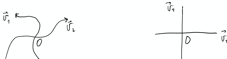
Figure 7: (Left) An example of non-straight eigenvectors \vec{v}_1 and \vec{v}_2 of a nonlinear map defined by (34). (Right) An example of eigenvectors \vec{v}_1 and \vec{v}_2 of a linear map defined by (35).
