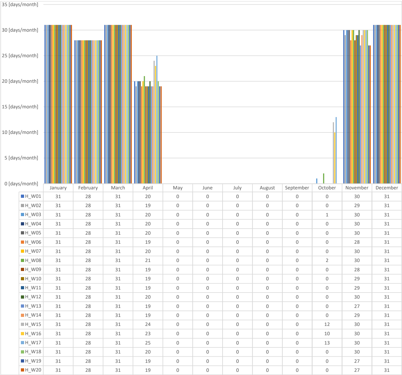
Figure 4. Comparison of the number of heating days needed to obtain the set point temperature, as a function of the stratigraphies.
