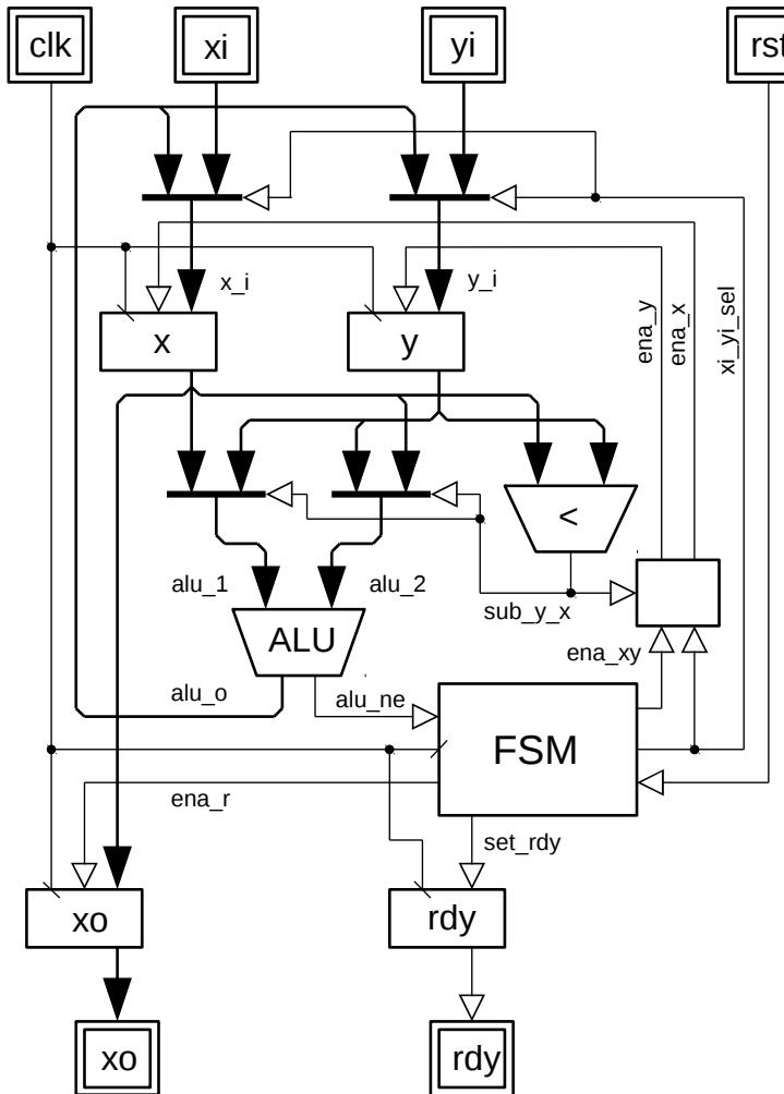
Register-transfer level description with comparator controlling subtractions.
