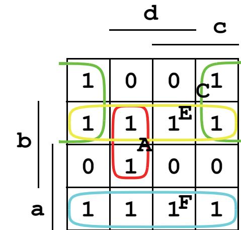
$$f = b \bar{c} \bar{d} + \bar{a} \bar{d} + \bar{a} b + a \bar{b}$$
