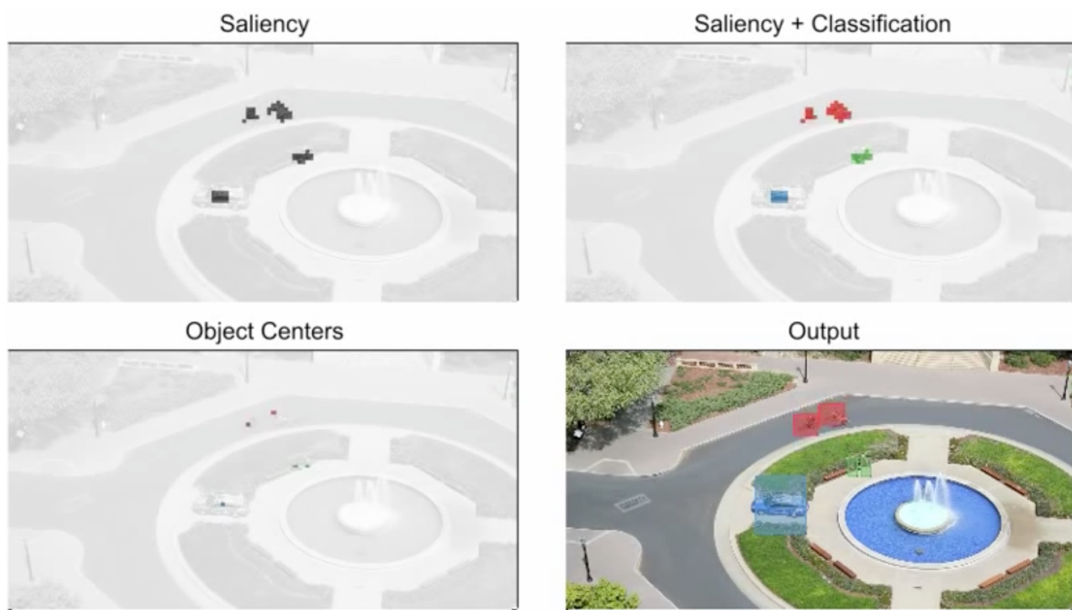
Fig. 2.5 Video feed recognition with TrueNorth chip [30]
