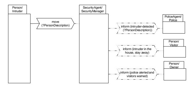
Figure 7: Interaction Frame Diagram of the Intruder Detection System
