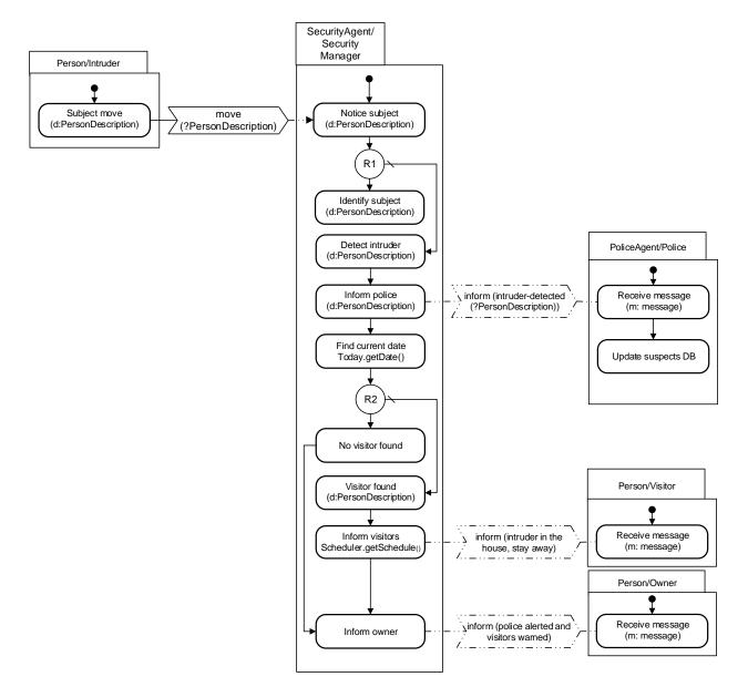
Figure 8: Behaviour Model of the Intruder Detection System
