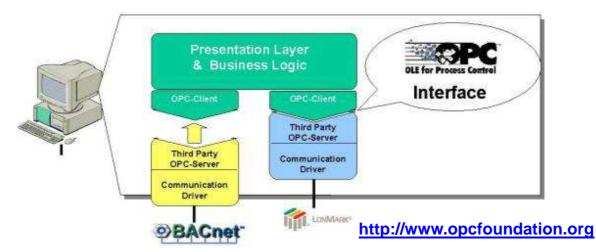
**Op**en **C**onnectivity standard for the secure and reliable exchange of data between devices and software's from multiple vendors
